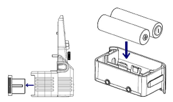
To replace the batteries, separate the battery tray from the pump: unscrew the screws on the front and pull the battery tray out of the unit.
